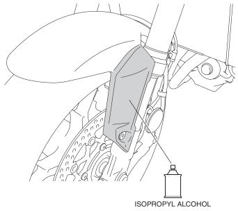
3. Peel off the adhesive backing on the left front fender panel as shown.
