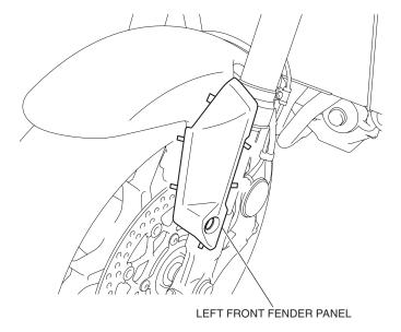
5. Remove the adhesive backing as shown.
