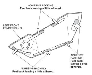
4. Attach the left front fender panel as shown.
